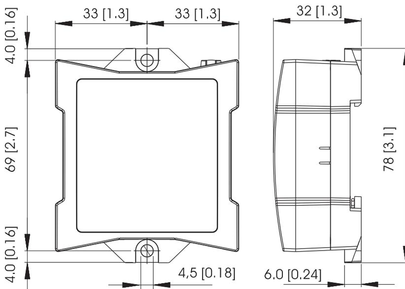
Figure 5: Dimensions in mm [inch]
