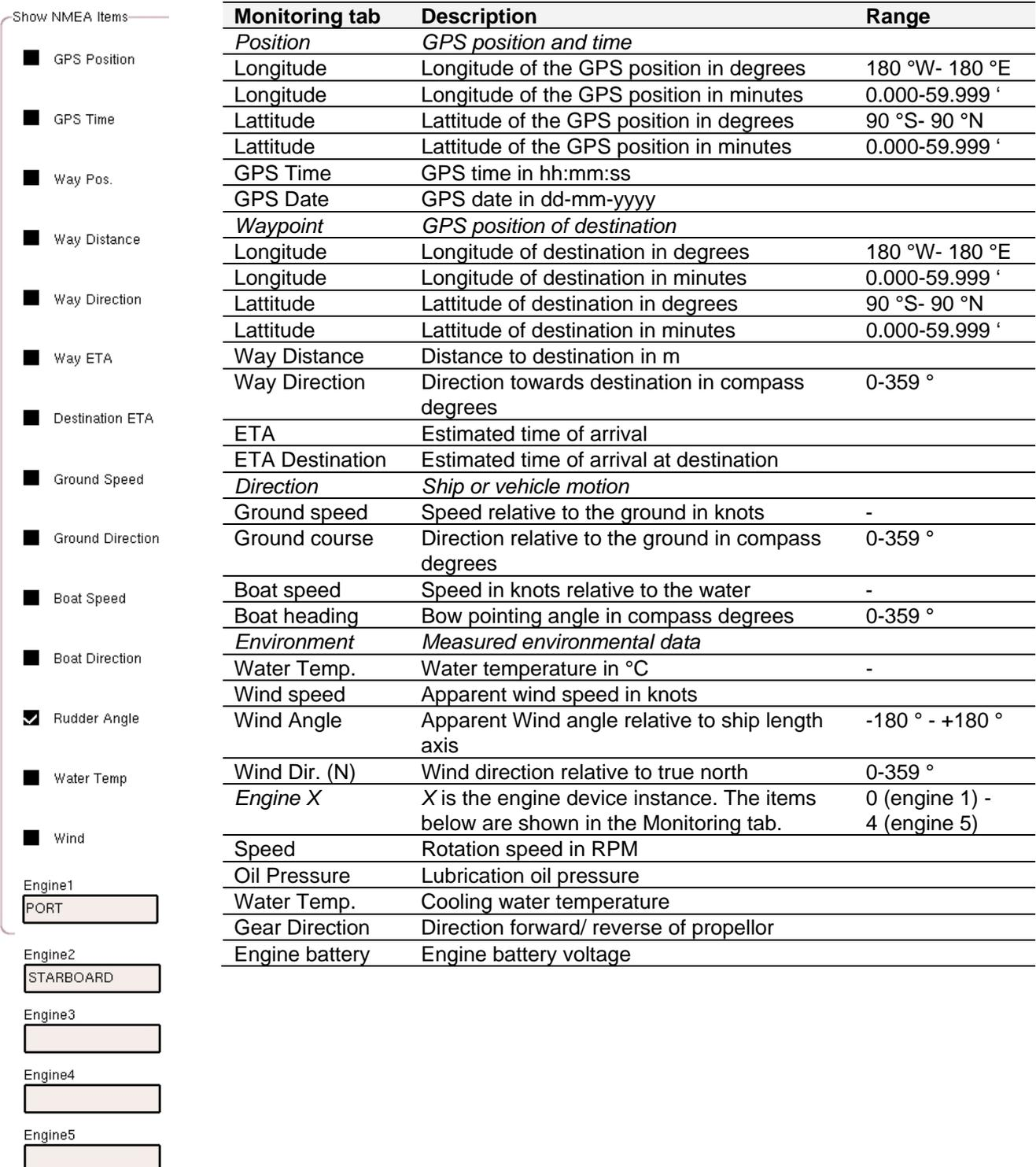
Figure 1: NMEA items available for MasterBus, table with MasterBus monitoring items
