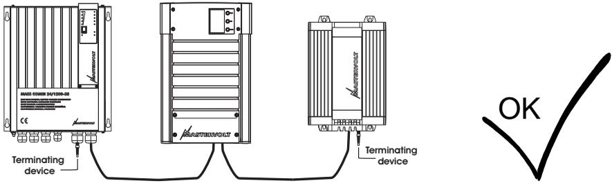
The electric power for the network comes from the connected devices.
