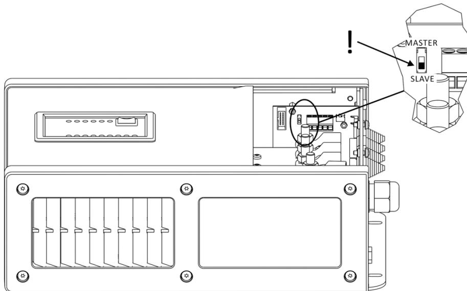
The rotary selector switch of a slave acts as an 'address' selector now. Each slave should use a unique address number. Since a maximum of 6 chargers (1 master and 5 slaves) are allowed in a parallel system, addresses 0, 1, 2, 3 and 4 can be selected. So when a parallel system of 3 battery chargers is installed, slave 1 should be set to address '0' and slave 2 to address '1'. Please see the image below for the location of the rotary selector switch of a slave charger set to '0'.
