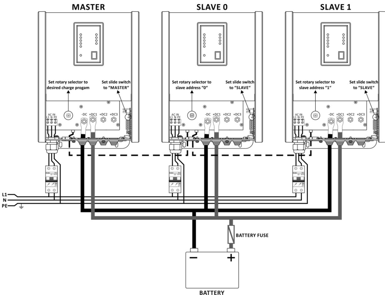
When the charger system is controlled by a Universal Remote Control, a Basic Remote Control or is configured/monitored by TBS Dashboard, please make sure that these connections are always made to the master battery charger. The same applies to the battery temperature sensor. Please see the image below for details:
