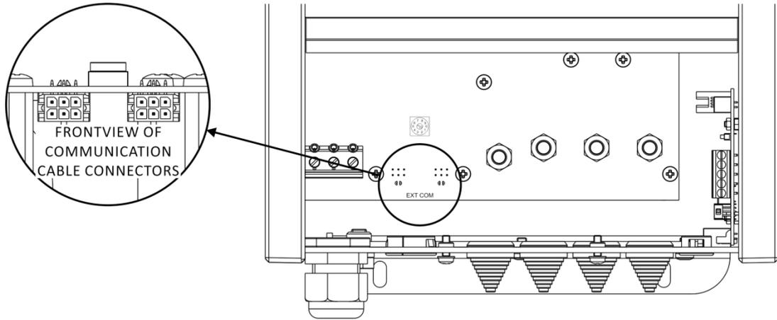
You are allowed to use any of the two communication cable connectors, since these are wired in parallel on the PCB anyway. Once the parallel communication cables are installed, we can start making the AC and DC connections.
