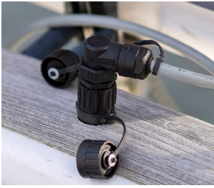
[Figure 4 ] Feedthrough connectors installed in the boat
