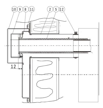
Make a ø90 mm hole to the wall, whose midpoint is at a height of 225 millimetres from the bottom of the heater.
