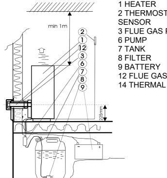
1 HEATER 2 THERMOSTAT TEMPERATURE SENSOR 3 FLUE GAS PIPE 6 PUMP 7 TANK 8 FILTER 9 BATTERY 12 FLUE GAS WALL SLEEVE 14 THERMAL INSULATION
