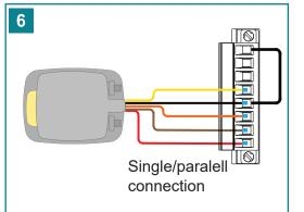
On the Battery Safety Connector, move the jumper wire to pins 4 & 8. Connect the ML Switch wires to the Battery Safety Connector according to the detailed figures in the user manual of the MLI Ultra.
