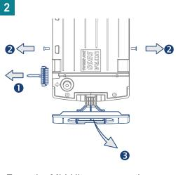
From the MLI Ultra, remove the Battery Safety Connector (1) and on either side the bolt closest to the positive terminal (2). Tilt the positive (right) side handle (3).
