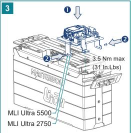
Place the bracket over the MLI Ultra (1), aligning the bracket holes with the holes of the bolts. Tighten the bolts back in place (2). 14.7 to 19.6 Nm (130 to 170 In.Lbs)
