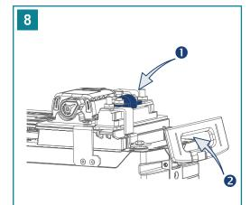
Remove the clear fuse cover and install the T-fuse (1). Place the cover back on the fuse holder. Close the side handle as much as possible (2). It will not close completely.
